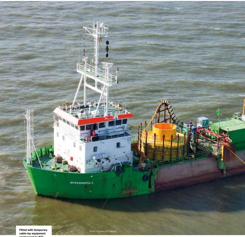
cable lay equipment engineered by KCI, Tideway's Pompeï installed 14.1 km from the Scheveningen shore to an oil production platform.
